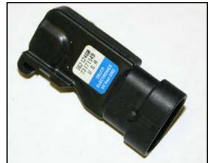
The Manifold Absolute Pressure sensor attaches to the harness with Connector J17.
