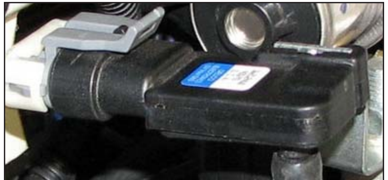
The Manifold Absolute Pressure sensor attaches to the harness with Connector J17.
