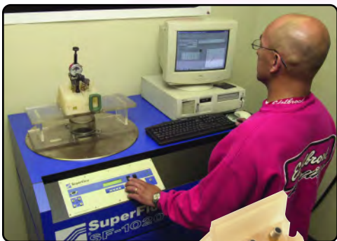
Edelbrock engineers test a cylinder head "flow box" on our SuperFlo SF-1020 flow bench.
