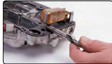
Checking float level with a 7/16" drill bit
