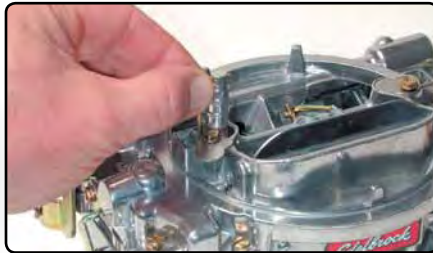
Metering rods can be changed without removing the lid from the carburetor
