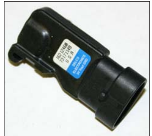
The Manifold Absolute Pressure sensor attaches to the harness with Connector J17.
