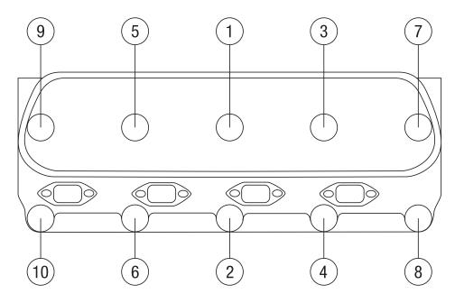
Figure 1 - Small Block Ford Cylinder Head Bolt Torque Sequence Torque Bolts in 3 to 4 Steps, Gradually Approaching Final Torque (See "Specifications" Below for Head Bolt Torque Spec)
