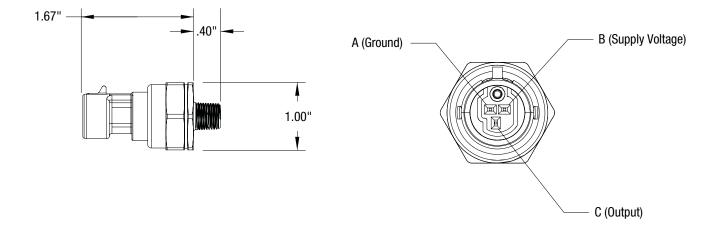
Figure 2 - Sensor Dimensions
