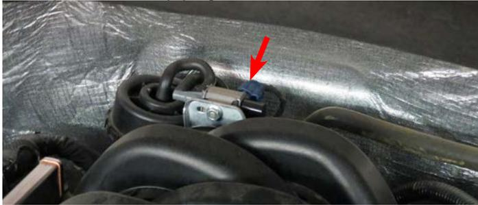
32. Using an 8mm socket, loosen the remaining six (6) intake manifold bolts. Note: Bolts can not be removed from manifold. Loosen enough so threads are disengaged from the cylinder head.
