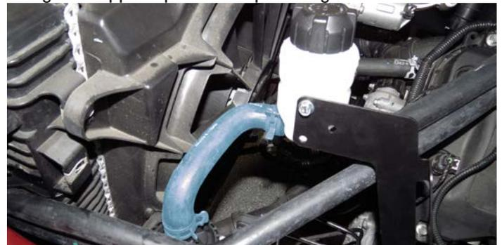
82. Install supercharger to LTR hose using the supplied pinch clamps in bag #3 and route through radiator shroud as shown.
