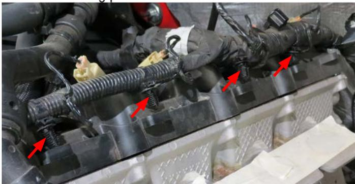
60. Completely Remove the square coil harness retaining tabs located on the top of both valve covers. File down any rough edges. Also, trim off the top of the rear round edge of the passenger side valve cover. Carefully remove all debris with a shop vac.
