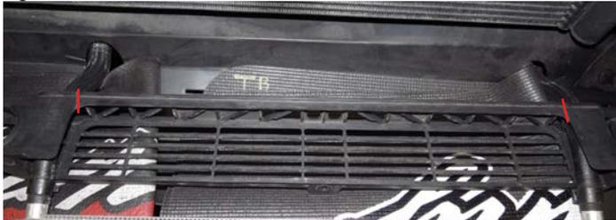
89. Install the LTR brackets by first removing the plastic push pins in locations #1, #3 and #4. Orient the brackets as shown below and secure with the supplied hardware. Leave hardware slightly loose for adjustment later. **Note: The brackets should be mounted under the rubber radiator shroud. The bolt and washer will hold the shroud and bracket in place. All hardware is located in bag #3.**
