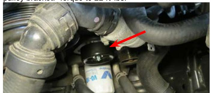
58. Using hose clamp pliers, remove factory coolant bleed hose and discard. Use the factory clamps to install the included hose show below.
