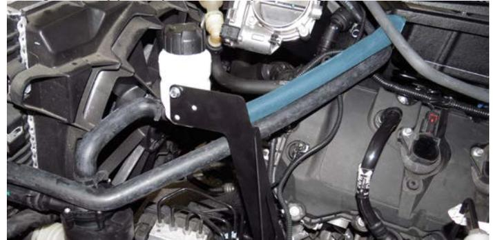
81. Install the surge tank to water pump hose as shown using the supplied pinch clamps in bag #3.
