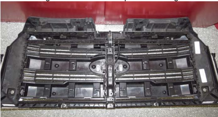
108. Reinstall the grille and radiator cover using the factory hardware and the two, new push pins that secure the air scoop as shows below. **Be sure to reconnect the grill shutter harness even though this feature is no longer used.**
