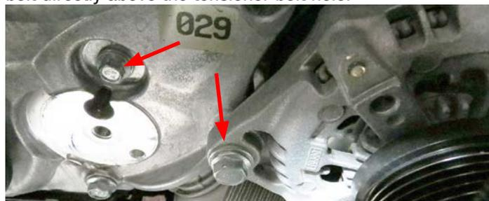
54. Using the bolts supplied in Bag #2, secure the small idler bracket by installing the M10 x 110mm bolt through the ear of the alternator, the M8 x 90mm bolt into the top front cover hole and the M10 x 45mm bolt through the center hole that was used to secure the stock tensioner. Torque M10 x 110mm bolt to 32 ft/lbs and the other two bolts to 22 ft-lb.
