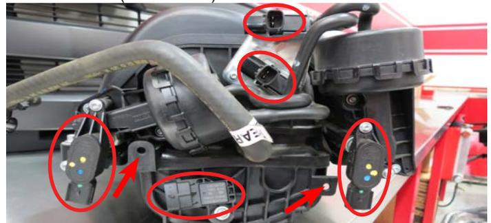
36. Make sure the IMRC harness is completely disconnected from above locations and remove the manifold. Clean the cylinder head surfaces and tape off intake ports so nothing can mistakenly fall into any of the cylinders.
