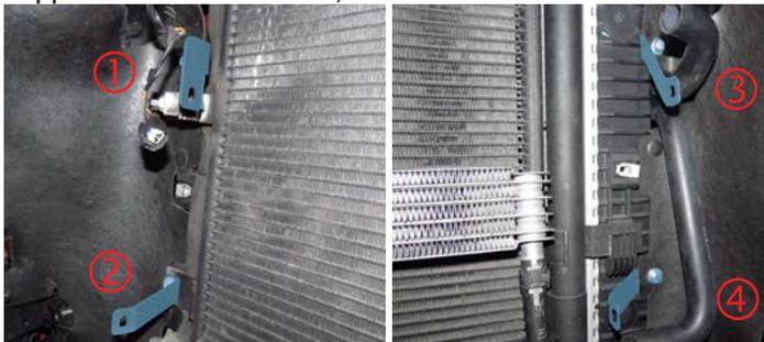
90. Using the measurements below, insert the plastic ties through the LTR fins in these locations from back to front. **DO NOT DRILL. Press in by hand ONLY.**
