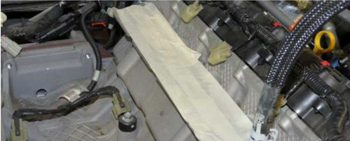
37. Tape up the four (4) IMRC harness plugs at the plug ends and secure plugs to the main harness out of the way. These will not be reused.
