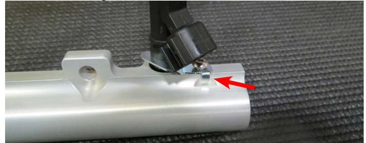
70. Install the fuel rails and secure using four (4) SHCS M6 x 16mm screws from Bag # 1. **Start fuel rail bolts BY HAND first and make sure thread engagement is smooth before tightening with tool.**
