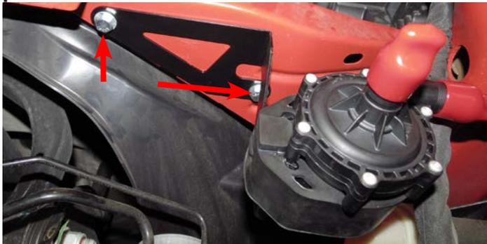
79. Remove the indicated strut tower nut and install intercooler reservoir bracket over stud. Loosely tighten the strut tower nut. Using the supplied M8 x 20mm bolt, washers and nut located in bag #3, fasten the bracket to the hole on the back of the control arm mount. Install intercooler overflow tank on bracket using the supplied M6 x 10mm bolts and align bracket so tank is sitting upright. Tighten all hardware. **Do not overtighten bolts securing tank to bracket.**
