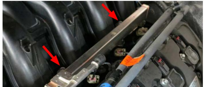
31. Disconnect the two (2), blue IMRC solenoid harnesses from the back of the intake manifold by pushing down on tab and pulling plug out. The second plug (not shown) is directly below the top plug.
