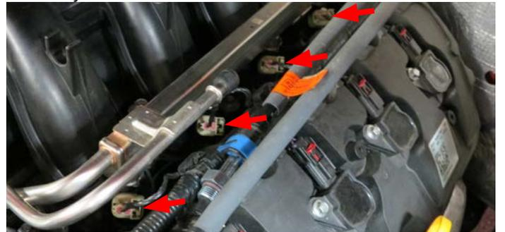
30. Using a 10mm socket, remove four (4) fuel rail bolts (driver side shown). Firmly and evenly lift up on fuel rail from both sides and remove from intake manifold.
