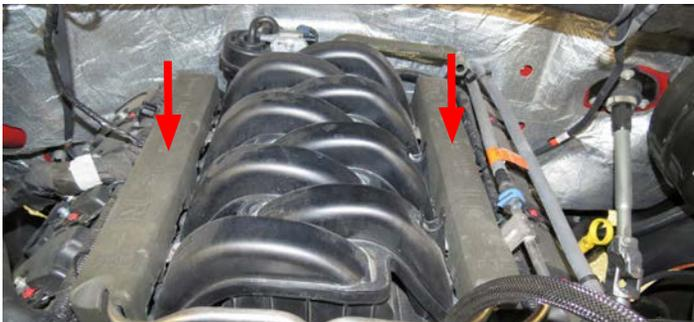
28. With the vehicle **COMPLETELY** cooled. Put rags under the fuel rail fitting and remove the fuel line from the rail by pulling the blue locking tab up. Cap off the fuel rail and fuel line with appropriate cap and plug to prevent spillage. Clean up and spilt fuel before proceeding.
