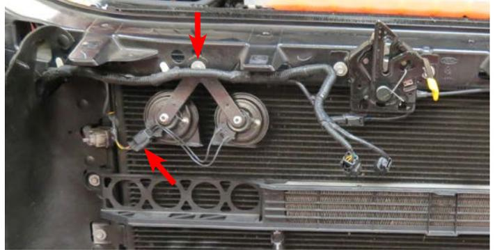
85. Disassemble the horns from the factory bracket and reinstall on the included, new bracket as shown.
