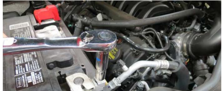
14. Drain the coolant by loosening the petcock located on the driver side of the radiator. **TIP: Placing a hose onto the drain spout will reduce potential coolant spillage.**
