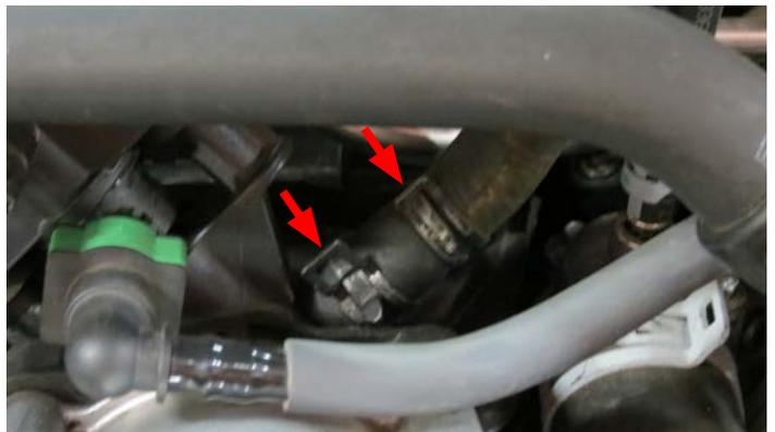
24. Disconnect the evap line from the purge valve by squeezing the green clip together at the bottom and lifting the tab up. Disconnect purge valve harness by pushing down the black tab and pulling plug out.
