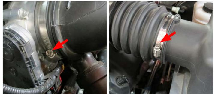
21. Remove the brake aspirator and driver side PCV hose from the back of the intake tube. Remove PCV hose from driver side valve cover and set aside. **TIP:** The brake hose is removed by pushing down the yellow clip and pulling out on connector. The PCV hose is removed by pushing out on the grey tab and pulling the connector out.
