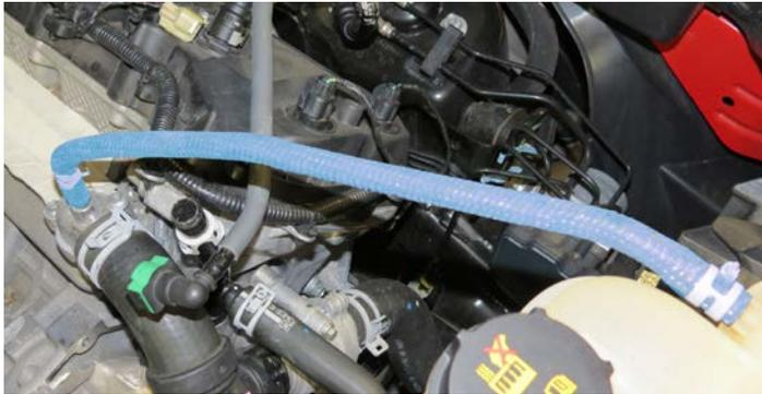
59. Using a panel removal tool, remove the engine harness from both valve covers. Using wire cutters, carefully cut wire harness retaining pins from the harness and discard.
