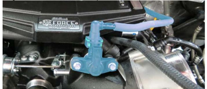
75. Using an 8mm socket, remove the throttle body from the stock manifold and install it onto the supercharger manifold using the supplied O-ring gasket, factory bolts and included extension harness.
