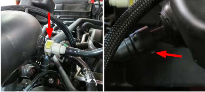
22. Remove the air box bolt using a 13mm socket. Remove intake tube and air box assembly from truck. The air box and tube will not be reused. Save the factory bolt.
