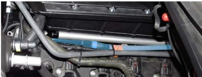
73. Reinstall the heater hose by installing the hose connector onto the fitting first, then tuck the hose under the supercharger lid.
