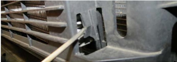
88. Cut a slot on each side of the trans cooler bracket where the red lines are drawn below. Remove the bracket from the hoses and discard. Carefully prop the trans cooler up and against the A/C condenser.
