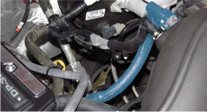
105. Verify that the coolant petcock is closed, then refill the coolant system. Use of a vacuum filler is recommended.
