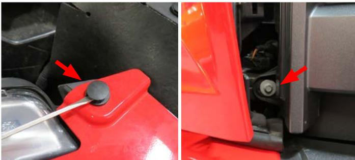
18. Remove six (6) push pins securing the flexible radiator shroud to the grille (3 pins per side). Tip: The two (2) lower pins (not pictured) can be removed by hand carefully if tool is not accessible.
