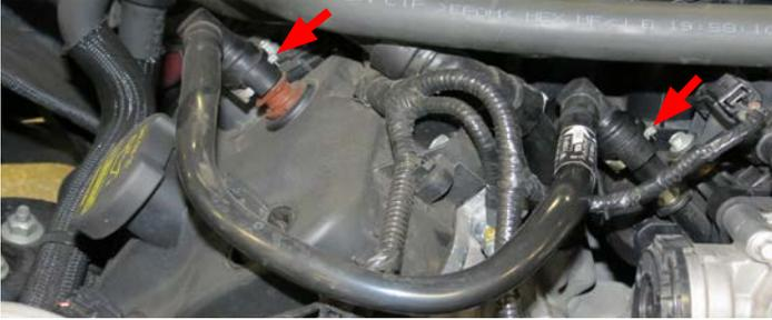
26. Disconnect the throttle body harness by pulling the red locking tab out and push down on the black tab as you pull the plug out.
