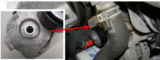
39. Using a 3/8" breaker bar or equivalent, release the tension from the secondary A/C drive tensioner and remove the A/C drive belt and discard.
