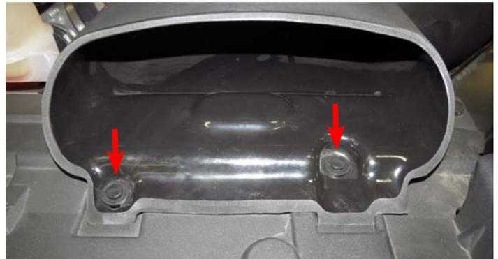
109. Secure the head light fascia by carefully pushing it back into place and reinstall the factory push pins.
