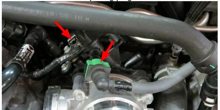
25. Remove the passenger side PCV hose by pushing the grey tabs out and pulling up on the connectors.
