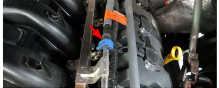
29. Unplug the eight (8) fuel injector connections (driver side shown) by pushing down on the tab and pulling plug out of injector.
