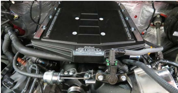
66. Secure the supercharger manifold to the cylinder heads using a 10mm swivel socket to install ten (10) M6 x 30mm intake manifold bolts supplied in hardware Bag # 1. Using the torque sequence below, torque the bolts to 8 ft-lbs.
