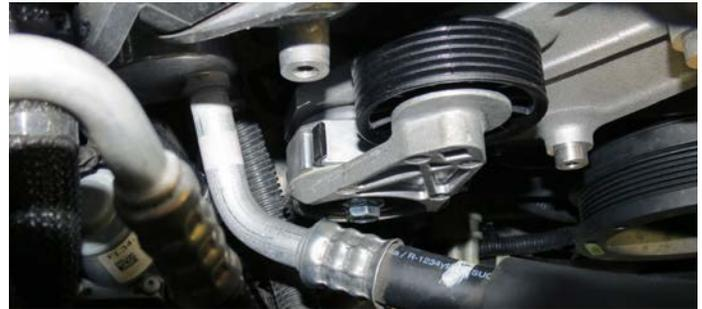
56. Install two (2) idler pulleys, one (1) 76mm and one (1) 70mm, with two (2) M8 x 20mm bolts and washers from bag #2. The smaller 70mm pulley should be installed on the uppermost boss on the tensioner bracket. Torque both idler pulley bolts to 22 ft-lbs.
