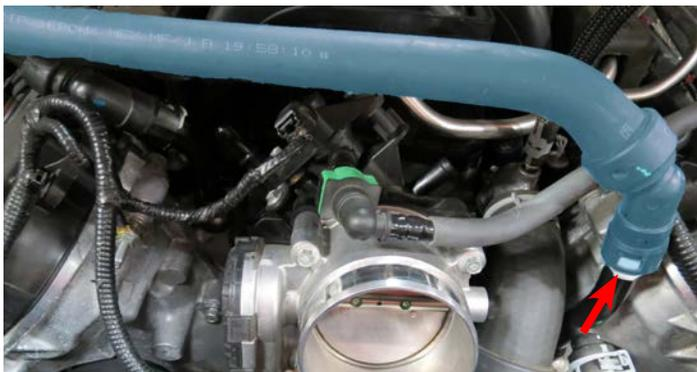
34. Lift the intake manifold and rotate counterclockwise as shown below. Locate the driver side IMRC position sensor harness and disconnect by pulling out the red locking tab, pushing down on the plug's clip and pulling the plug out. At this time, disconnect the MAP sensor harness located to the right of the driver side IMRC sensor. **See step #35 for plug locations.**
