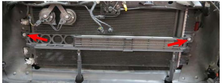
87. Pry out the clips on both sides of the transmission cooler bracket and slide the bracket down toward the cooling hoses.
