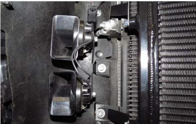
96. Install the intercooler pump/evap relay using steps A-D (harness ends are labeled for your convenience). **Note: All wires should be clear of any moving or potentially hot surfaces. Secure wires in a safe position with wire ties as necessary.**
