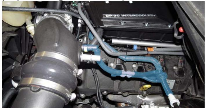
104. Using the factory 45° fitting on the valve cover and the remaining 90° fitting from the passenger side PCV line, Assemble the new driver side PCV line with the supplied length of 1/2" hose as shown.
