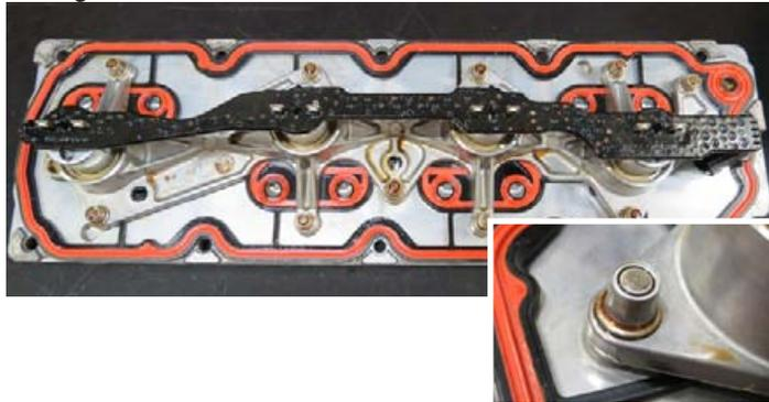
44. Using a cutoff wheel or equivalent, cutoff eleven (11) rivets securing the solenoid assembly onto the valley tray. Be careful not to damage the gasket as it will be reused.
