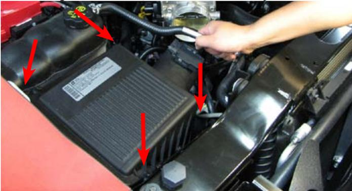
119. Replace the factory air filter with the supplied Green reusable air filter.
