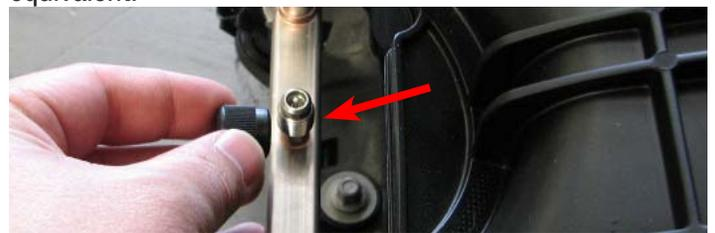
32. Remove the fuel hose safety clip, then remove the fuel supply line using a 3/8" Fuel Line Removal Tool.
