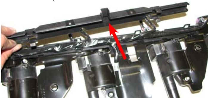
38. Remove the factory valley tray, by unplugging the oil pressure sensor and the Active Fuel Management (AFM) system (if applicable). Use a 27mm wrench to remove the oil pressure sensor from the valley tray. Unbolt the eleven (11) bolts securing the valley tray using a 13mm socket.
