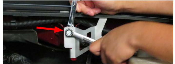
134. Tighten the ball joint adapter using a 14mm ratchet and install the hood prop onto the ball joint adapter.
