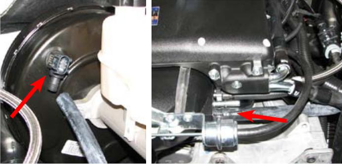
106. Install the driver side PCV hose by sliding it onto the rear barb located on the driver side valve cover. Then install it on the center barb located on the manifold nose. Be sure to route the hose between the coil bracket and intercooler hose.
