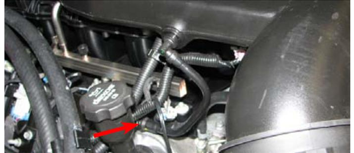
22. Using a 15mm socket and a breaker bar, remove the serpentine belt by rotating the tensioner clockwise until the belt can slide off the idler pulley.
