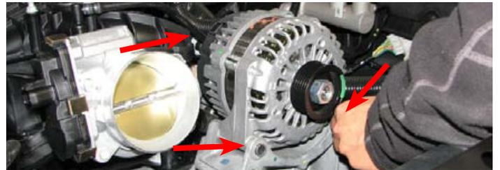
24. Remove the idler pulley on the alternator bracket using a 15mm socket.
