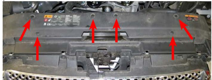
16. Using a 10mm socket, remove the six (6) top support bolts securing the fascia.
