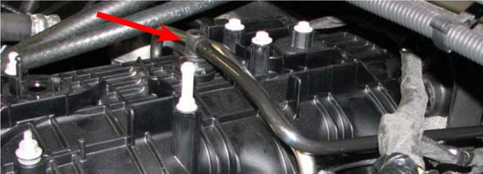
27. Disconnect the EVAP solenoid hoses and unplug the EVAP harness. Then unplug the MAP harness from the MAP sensor and ETC harness from the throttle body.
