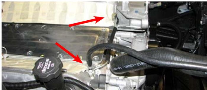
66. Using a razor blade or equivalent, remove the rubber guard on the factory coolant crossover and install it onto the supplied coolant crossover.
