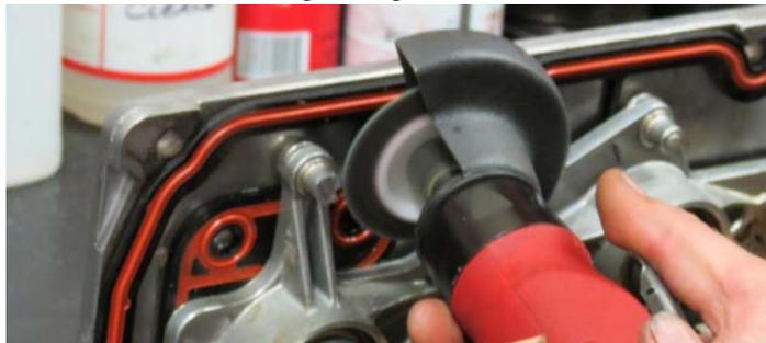
45. Remove the solenoid assembly from the valley tray and carefully remove the gasket.
