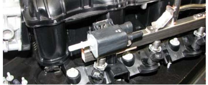
103. Install the supplied EVAP bracket onto the driver side coil pack assembly stud using one (1) M6 nut from Bag #2. Stud location is in between the first and second coil packs. Install the factory EVAP on to the EVAP bracket as shown.
