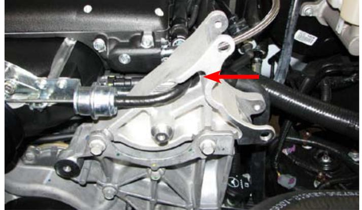
108. Remove the bolt, washer and bushing from the stock 90mm pulley and install them on the supplied 76mm pulley.
