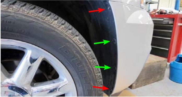
18. Using a 10mm socket, remove four (4) bolts from the bumper/fender support brackets. Two (2) from the driver side and two (2) from the passenger side.
