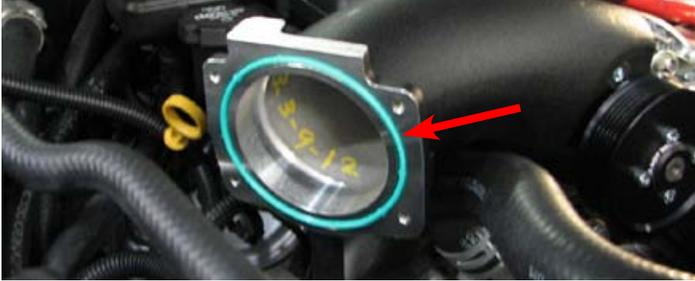
117. Using four (4) supplied M6 x 40mm bolts in Bag #1, install the factory throttle body onto the throttle body flange.
