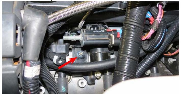
104. Install the factory EVAP hose to the rear barb of the EVAP solenoid. Install the provided EVAP hose on the right rearmost barb of the manifold nose and connect it to the front barb of the solenoid. DO NOT connect the EVAP harness to the solenoid.
