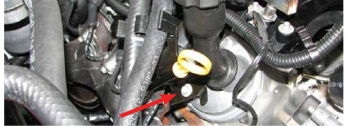
30. Disconnect all eight (8) injector plugs (four driver side, four passenger side).
