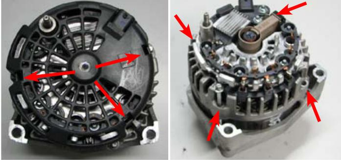
111. Clock the rear portion of the alternator clockwise one bolt position so that the harness plug points at the right mounting hole. Apply red Loctite to the bolt threads and reinstall the four (4) alternator bolts and plastic cover.
