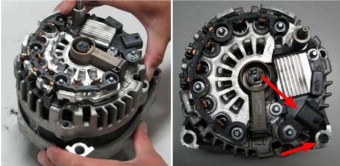
112. Using a 15mm socket and the supplied M10 x 90mm bolts in Bag #1, install the alternator onto the new alternator bracket and torque to 41 ft-lbs (55 Nm). Re-connect the alternator harness plug.
