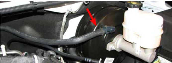
29. Using a 10mm socket, remove the bracket securing the heater hoses.
