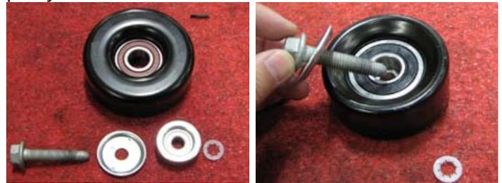
109. Apply Red Loctite to the threads on both idler pulley bolts. Then use a 15mm socket to install the 76mm idler pulley with the factory hardware to the left idler pulley location. Install the additional idler pulley to the right idler pulley location with one (1) M8 x 20mm bolt and one (1) M8 washer from Bag #1. Verify that both pulleys spin freely.
