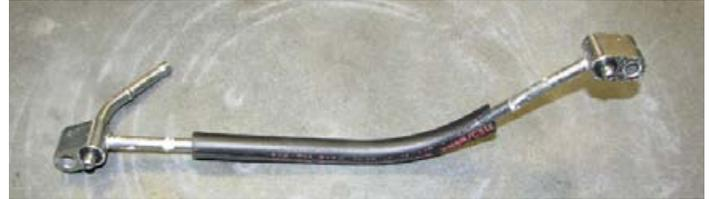
67. Using a 10mm socket, install the supplied coolant crossover using the factory bolts, making sure the inlet port is on the driver side. Reinstall the factory coolant feed hose to the crossover.
