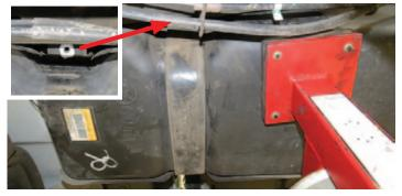
5. Lower the fuel tank slightly. Loosen the fuel fill pipe clamp at the fuel tank and remove the fuel fill pipe from the fuel tank.
