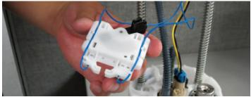
22. Install the sending unit onto the fuel pump module. Make sure the sending unit wires do not get pinched between the sending unit and the fuel pump module.
