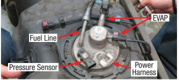
10. Move the fuel line, EVAP lines and harness away from the fuel pump module.
