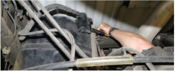
4. Place an adjustable jack under the fuel tank for support. Using a 15mm socket, remove both fuel tank strap bolts and straps.
