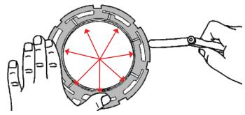
19. If warpage is less than .41 mm (.016 in), the lock ring does not require replacement. If warpage is greater, the lock ring must be replaced.
