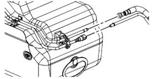
3. Disconnect the fuel tank EVAP line from the EVAP canister. Cap or tape up the fuel and EVAP lines to prevent possible system contamination.
