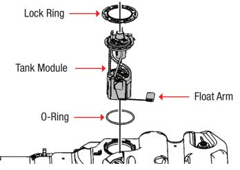
**NOTE:** Some lock rings were manufactured with "DO NOT REUSE" stamped into them. <u>These lock rings may be reused if they are</u> not damaged or warped.
