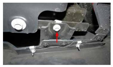
19. Remove the grill/bumper cover. Start in the middle and loosen the cover from the core support. Then, gently start pulling the bumper out and down, taking care not to break the plastic guide pins beneath the headlights. Unplug foglights if equipped.
