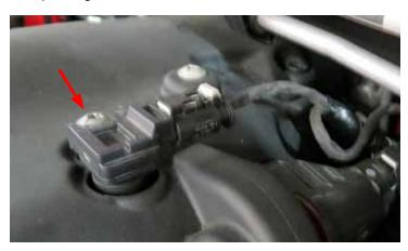
39. Disconnect the EVAP solenoid connections and then remove by using a 10mm socket as shown. This EVAP and bolt will be reused on the supercharger later.
