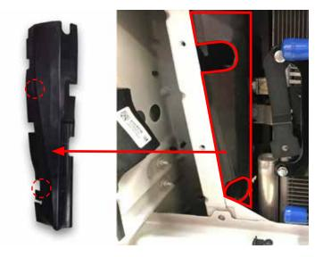
24. Reinstall the plastic cowl and install the LTR brackets (Shown in red) by reusing the bolts that were removed when uninstalling the shutters assembly. NOTE: PEM nuts face towards rear of vehicle.
