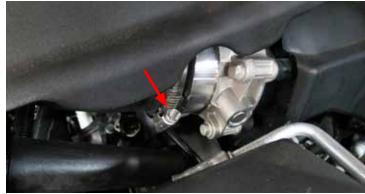
37. Unplug the harness from the throttle body. Using a 10mm socket, remove the throttle body.
