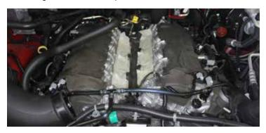
44. Using a 13mm socket, remove the front engine cover bracket. Renstall the original bolt in the passenger side.
