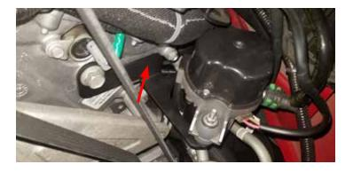
51. The new TMAP sensor is pre-installed from Edelbrock. A TMAP extension cable is included. Once the intake is installed, the TMAP will be difficult to access.
