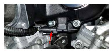
66. Install the throttle body to the supercharger nose using the factory hardware and supplied O-ring. O-ring lube is recommended. Connect Throttle Body extension and the throttle body control cable.
