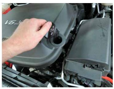
36. Disconnect the intake tube from the throttle body and lift the engine cover up. Disconnect the PCV hose from under the front right of the cover. The cover should be free now. Replace oil cap when finished.
