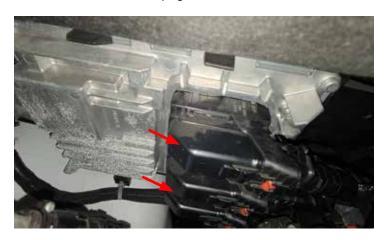
4. Lift up on the 2 tabs pictured below while pulling the ECU out from the top.
