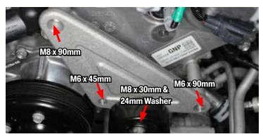
50. Attach the new vacuum pump bracket to the timing cover using the original bolt on the left side and original hardware on the right side. Reattach the pump on the new bracket and reattach all plugs and hoses.
