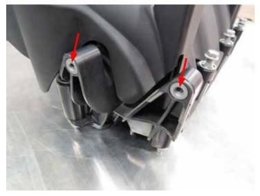
42. Underneath the throttle body flange, remove the 10mm bolt on the driver's side of the vehicle as pictured.
