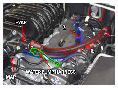
74. Install the 12 volt constant power lead on the Water Pump Harness as pictured here.
