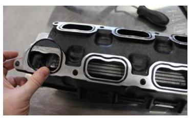
53. Remove the intake port covering. Clean the sealing surface and check for any stubborn dirt or debris before proceeding.
