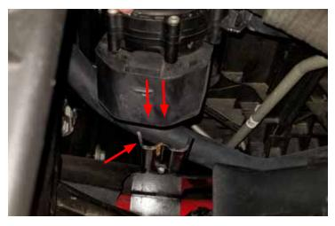
32. Disconnect the PCV hose and air intake from the engine cover.
