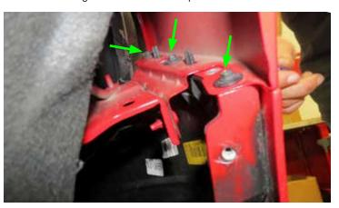
14. Using a T15 screwdriver, remove all 6 screws on top of bumper cover.
