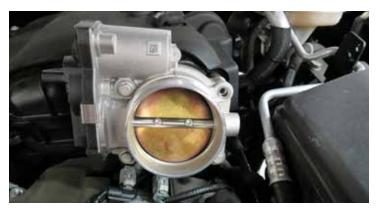
38. Using a T25 screwdriver, remove the MAP sensor and disconnect the cable. Set the MAP sensor aside. It will be reinstalled on the supercharger.
