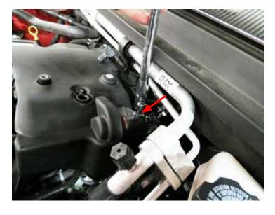
40. Using an 13mm socket and extension, loosen the 8 captive bolts holding down the intake manifold.
