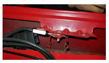
77. As you reinstall the panel, secure the relay by inserting the push-pin through the panel and then through the relay mounting tab.
