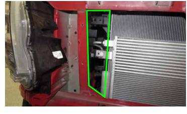
22. Carefully remove the plastic cowl on the passenger (right) side of
