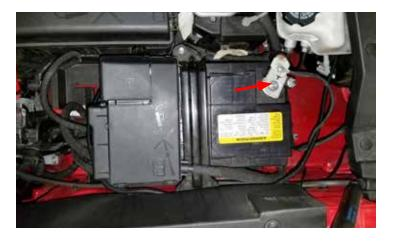
2. Using a 10mm socket, unbolt the coolant tank and move aside. Disconnecting the hoses is not necessary.
