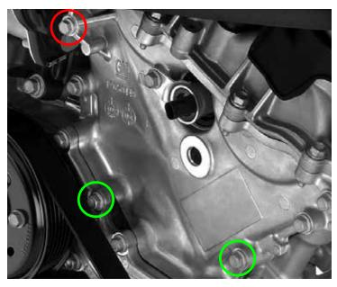
49. Attach the FEAD bracket and idler using the hardware provided in FEAD hardware bag #1 using blue Loctite.
