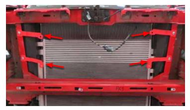
25. Install the Low Temp Radiator (LTR) to the brackets with the ports facing the passenger (right) side of the vehicle using the M6 x 16mm bolts from bag #2.
