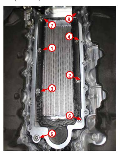
57. Place the gasket on the intake manifold base. Be sure to align the gasket with the holes to ensure a perfect seal.
