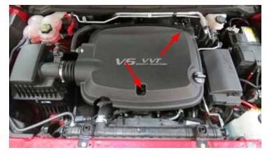
34. Using a 10mm socket, remove the bracket attaching the engine cover to the passenger side valve cover.
