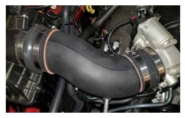
70. Reconnect the factory crank case ventilation hose to the bottom of the new intake tube.
