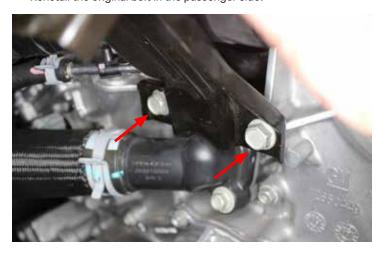
45. Remove the factory timing cover bolts (pictured) and install the wire harness support bracket using the original bolts.
