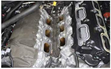
54. Before attaching the TMAP extension, feed the cable up underneath the factory lines as pictured. NOTE: You must connect the TMAP exention before setting the intake down into the valley.
