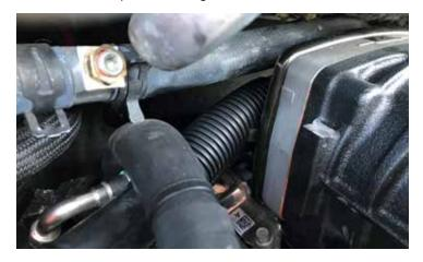
63. Using the hardware from bag #3, install the (8) M6 x 20mm on the sides, and (2) M6 x 16mm in the rear. Torque bolts 1 through 10 in the following order to 9lb/ft. (or 12Nm) of torque using blue Loctite. Install OEM MAP sensor behind the throttle body.
