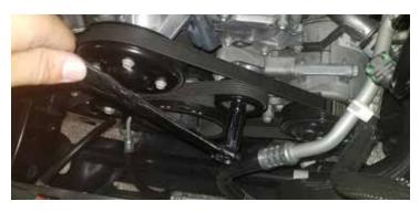
47. Disconnect the vacuum hose as pictured. Remove the bolts in the following picture and set aside. The bolts will be reused on the new bracket. The 13mm bolt has a nut on the opposite side. Be sure to recover this nut since it will be reused. Unplug and remove the vacuum assist pump and bracket from the front of the block, then remove pump from the OEM bracket.
