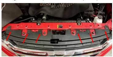
17. Remove (2) 10mm bolts from the center of the grill. NOTE: They are deep inside and can be hard to see. Do this for each side. NOTE: ZR2 models have (4) 10mm bolts.
