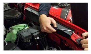
76. Remove the fender attachment bolt and secure the ground to the Water Pump Harness as pictured.
