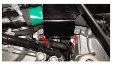
46. Using a 15mm socket, turn the tensioner counter-clockwise and remove the belt from the FEAD.
