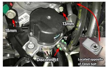
48. These 3 positions are where the new FEAD will be attaching. Remove the 2 timing cover bolts as pictured in green. The bolt circled in red was removed in step 44.
