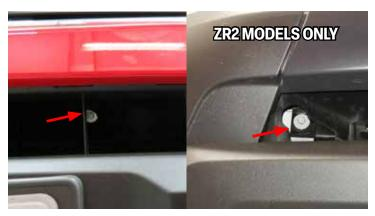
15. Remove the T15 screws (6 on each side) that attach the inner fender to the bumper cover. Do this for each side. NOTE: ZR2 models will need an additional T15 removed.
