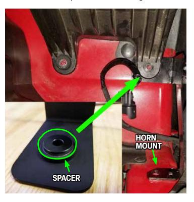
30. Replace the horn back into the same position on top of the forward water pump bracket strut using the same bolt that was removed. Reconnect the plug.
