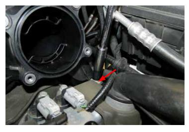
43. Once the manifold is removed, cover the intake ports to ensure nothing falls down into the ports.
