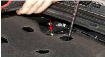
26. Uninstall the intake manifold by loosening (8) 13mm bolts and (2) 10mm bolts in the back. NOTE: The back two 10mm bolts are underneath the windshield cowl.
