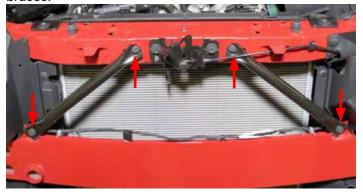
9. Using a 10mm deep socket, unbolt the horn assemble from the crash guard. Unplug the horns and set aside.
