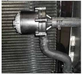
19. Install the rubber isolator onto the water pump bracket as pictured below.
