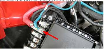
48. Remove the factory GROUND terminal nut attached to the chassis. Attached the GROUND connector on the water pump harness to the chassis ground and secure with the factory terminal nut. Remove the nuts securing the fuse box to the chassis. Gently remove the fuse box from the mounting studs and secure the relay to the mounting stud. Reinstall fuse box nuts.
