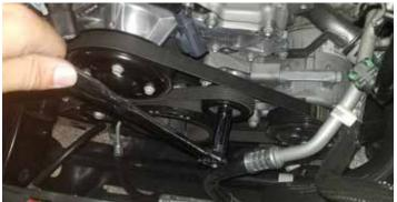
29. These 3 positions are where the new FEAD will be attaching. Remove the 3 timing cover bolts as pictured in red.
