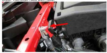
49. Route the EVAP connectors on the supplied water pump harness towards the EVAP solenoid. Install the water pump harness in-between the mating connectors on the EVAP solenoid and factory harness. TIP: Note connector orientation...
