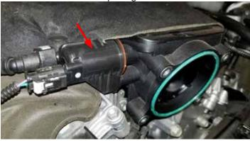
25. Uninstall the OEM MAP sensor located here. Set aside. This will be reinstalled.
