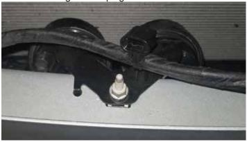
10. Detach the wire harness from the crash guard but leave the harness on the vehicle. Using a 13mm socket and extension, remove the 8 bolts holding the crash guard to the chassis. Detach any push clips that might be installed
