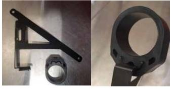
20. Install the insulator onto the pump. Attach the water pump harness and feed the harness through the radiator support towards the passenger side. Leave the bracket loose. We will come back to this once we reinstall the crash guard.
