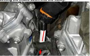
34. From bag #3, use the (7) M8 x 65mm bolts, and the (1) M8 x 30mm intake bolt in the back. Apply Blue Loctite to all. Use the following sequence to torque bolts 1 through 7 to 18 ft/lbs. Torque the #8 bolt (the short bolt) to 8 ft/lbs. Damage to intake may occur if torqued incorrectly.
