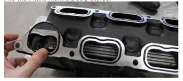
32. Remove the intake port covering. Clean the sealing surface and double check for any stubborn dirt or debris on the sealing surfaces before proceeding.
