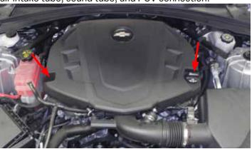
22. Remove the sound tube pictured here. Follow the tube back to the firewall and remove the 10mm nut. Rotate clockwise until the hose disengages and remove.
