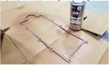
36. Place the gasket on the intake manifold base. Be sure to align the gasket with the holes to ensure a perfect seal.
