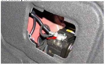
2. Using a 10mm socket, unbolt the fuse box and push aside. Disconnecting the wires is not necessary.
