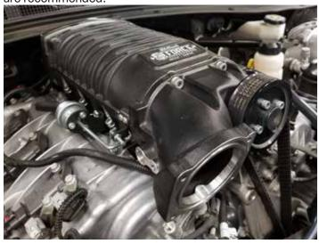
40. Using the hardware from bag #3, install the (8) M6 x 25mm on the sides, and (2) M6 x 16mm in the rear. Torque bolts 1 through 10 in the following order to 9lb/ft. (or 12Nm) of torque using blue Loctite. **NOTE:** Do not over-torque.
