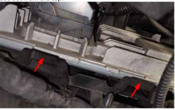
5. Once free, remove ECU and follow packing instructions. Be sure to include the HP Tuners RTD device with the ECU.
