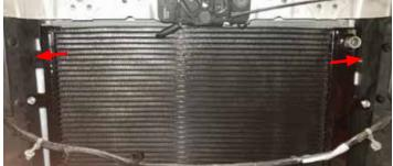
14. To secure the bottom of the LTR, drill 1/4" holes through the plastic cowl using the mounting tabs as a quide. Do once on each side.
