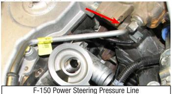
65. Use a 10mm socket to remove the bolt that holds the power steering line retention bracket onto the rack & pinion. Save this bolt, as it will be re-used.
