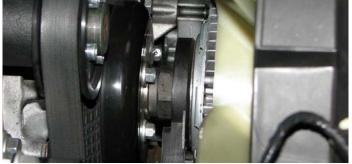
41. Use an 8mm socket to unbolt the thermostat housing and remove it. The housing, thermostat and 0-ring will all be reused.
