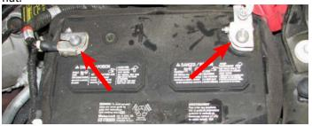
3. Use an 8mm socket to loosen and remove the positive battery terminal clamp, then tuck the wire aside.
