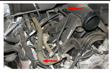
6. Use a 10mm socket to remove the inlet resonator bolt, then loosen the hose clamp and remove the resonator.
