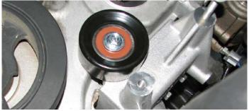
76. Tighten down the four mounting bolts, then tighten the pulley bolt. Verify that the pulley can spin freely once all the filter bracket bolts have been tightened.
