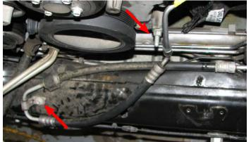
63. Use a 10mm socket to remove the bolt securing the power steering pressure line to the crossmember.
