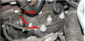
113. Mount the intercooler reservoir to its mounting bracket using the M6 x 16mm bolts supplied in Bag #5. Attach the molded Reservoir to Pump hose to the lower fitting of the reservoir; it must be routed down and around the radiator on the passenger side .Secure the hose with the supplied hose clamp.
