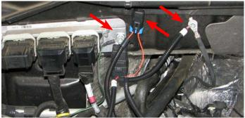
46. Mount the water pump fuse holder on the small bolt directly above the relay mounting location.
