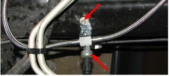
78a. For vehicles that utilize a power steering pressure sensor: Remove the sensor from the stock power steering line and install it in the new power steering hose then attach the wire harness connector.
