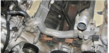
42. Use an 8mm socket to unbolt and remove the water crossover from the engine. Remove the gaskets on each end and retain them, as they will be reused. Then place making tape over each water passage.
