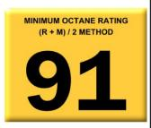
91 octane or higher gasoline is required at all times. If your vehicle has been filled with anything less, it must be run until almost dry and refilled with 91 or higher octane gasoline twice prior to installation.
