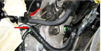
129. Connect the  $90^{\circ}$  end of the driver side PCV hose to the valve cover fitting. Connect the straight end to: the upper,  $90^{\circ}$  fitting, behind the throttle body flange, on the air inlet, next to the thermostat housing.
