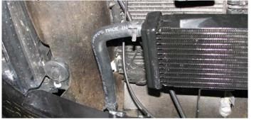
127. Attach water pump harness connector to the pump.
