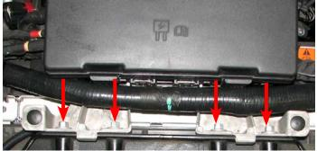
90. Route the alternator wire harness along the top of the radiator, working it below the fuse box support brackets, then plug it into the alternator.
