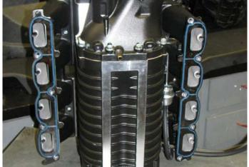
102. Lift the supercharger assembly, with the flange gaskets in place, over the water crossover and onto the engine. Insert the M6 x 30mm manifold bolts supplied in Bag #1 into their provisions to determine when the manifold is properly aligned.
