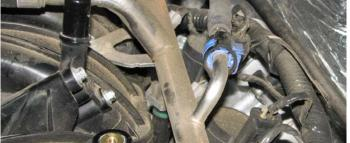
17. Disconnect the electrical connector from each of the fuel injectors.
