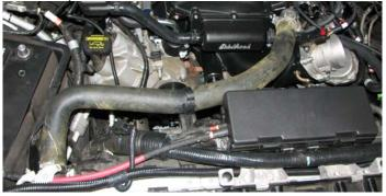
140. Remove the plastic sheet from the supercharger air inlet and install the throttle body O-ring supplied in Bag #1, on to the air inlet flange.
