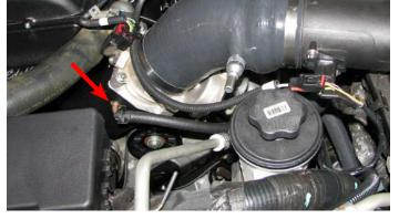
150. Verify that the coolant petcock is closed, then refill the coolant system.
