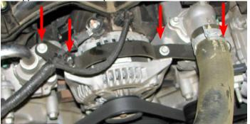
23. Remove the electrical connector from the alternator. Use a 10mm socket to remove the nut retaining the power wire. Remove the power wire and replace the nut. 24. Support the alternator while using a 10mm socket to loosen the two bolts that support the alternator. Lift the alternator off these bolts and set it aside. The two long bolts can be removed, as they will not be reused.
