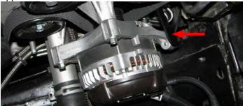
94. Remove the three bolts holding the belt tensioner in place, and remove the tensioner.
