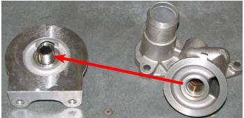
81. 2wd trucks should now install the oil filter on the new bracket, while 4wd trucks should refer to the instructions supplied with the #15834 kit
