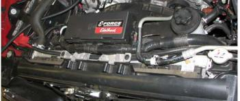
33. Un-clip the power steering hose from the top of the radiator. It is located on the drivers side.
