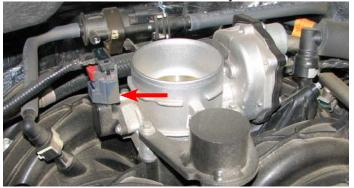
12. Use an 8mm socket to remove the two front throttle body bolts then remove the throttle body weight.
