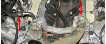
31. Use a screwdriver to remove the clamp that holds the heater hose to the water crossover then pull off the hose.
