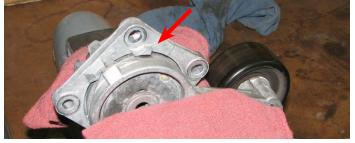
96. Use a grinding wheel or file to ensure that the area that was ground down is smooth and free of burrs.
