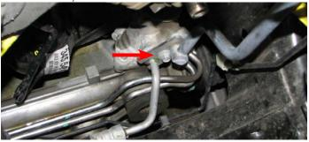
66. The power steering pressure line can now be pulled out of the steering box and removed from the vehicle.
